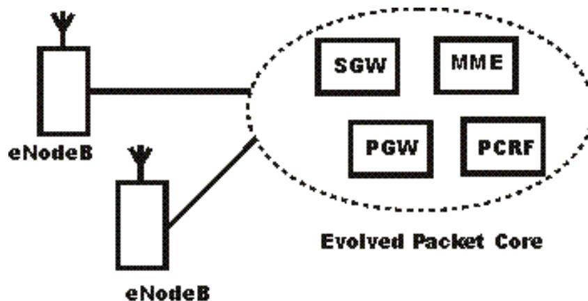
Fig: Elements of EPC – Evolved Packet Core
