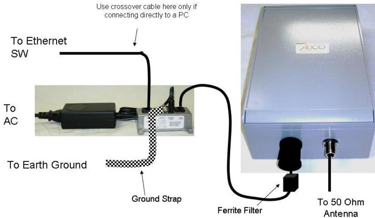
Figure 1 Connection Diagram
